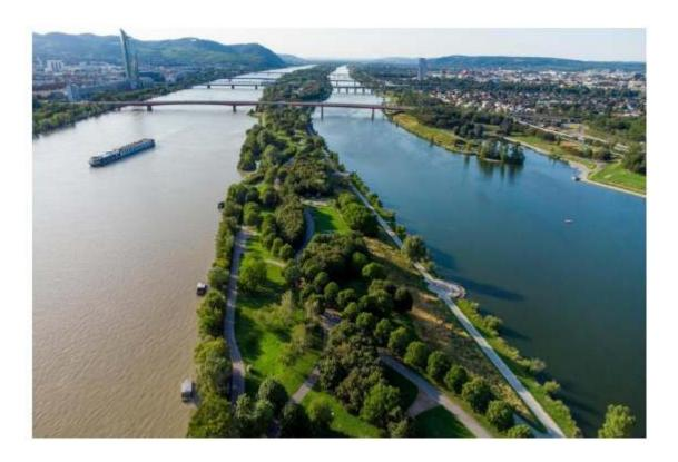
In Vienna, the Danube River running through the Austrian city has a channel constructed beside it to increase its capacity to hold rainwater in the event of a flood.
