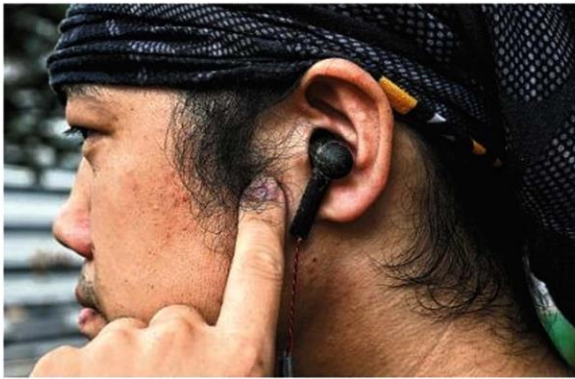
SMU PhD student Hu Changshuo testing the BreathPro earbuds, which have microphones that monitor whether a runner breathes in and out through his nose or mouth, as well as detect how his feet strike the ground.
