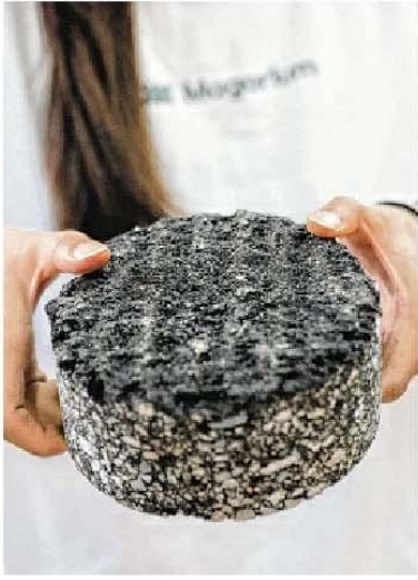
Above: A sample of asphalt premix made using NEWBitumen, a material used to build roads. NEWBitumen is made from unrecyclable plastic waste.
