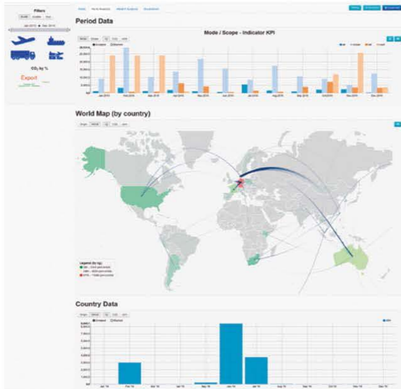
Screen grab from Carbon Dashboard 2.0, which uses advanced analytics and visualisation technologies to demonstrate where fuel is used and how emissions are generated
