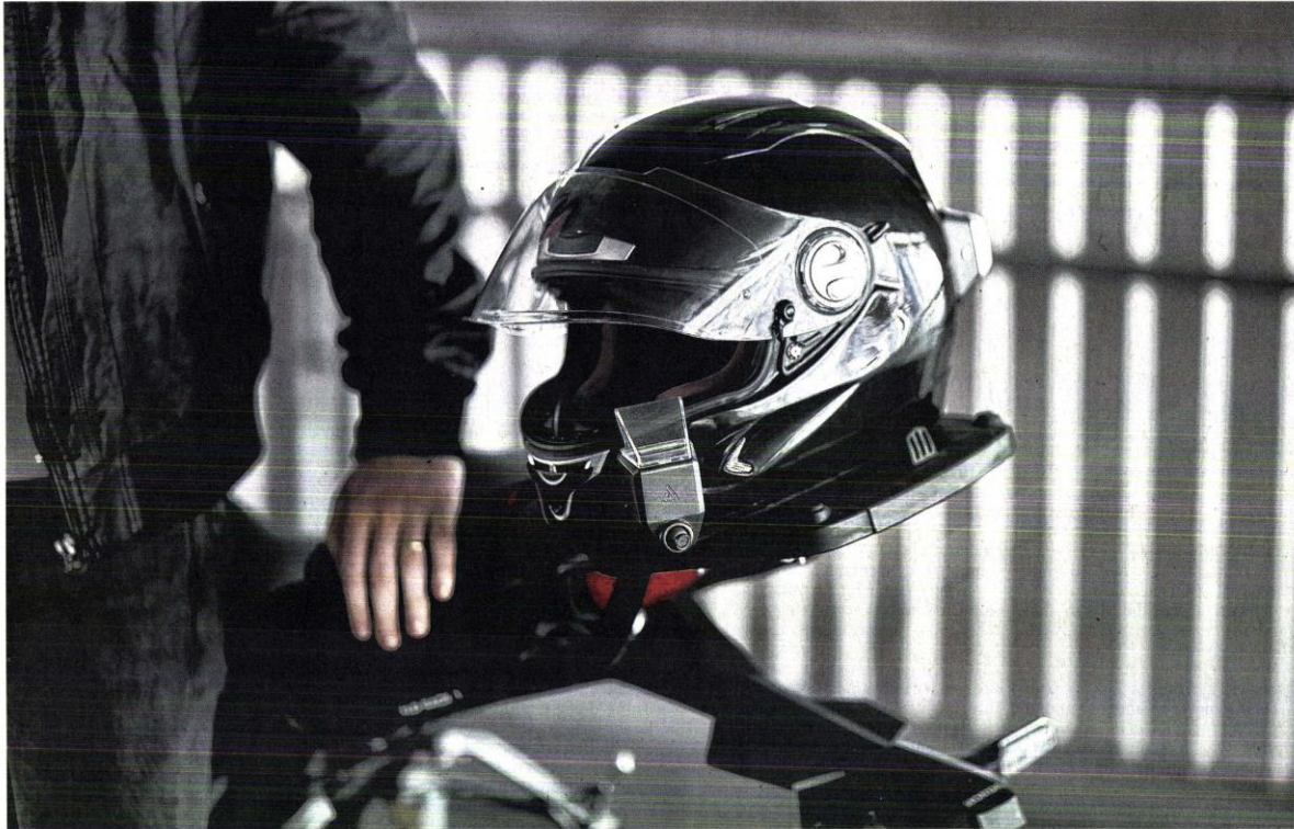
Argon Transform, which can be fitted to most helmets, has been touted as the world's first dual-camera smart helmet attachment. It consists of a rear-view camera, a front dash-cam with a heads-up display attachment and a handlebar remote control. PHOTO: WHYRE
