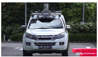
Autonomous vehicles in Singapore can be identified by the LiDAR sensors spinning furiously atop its roofs.
