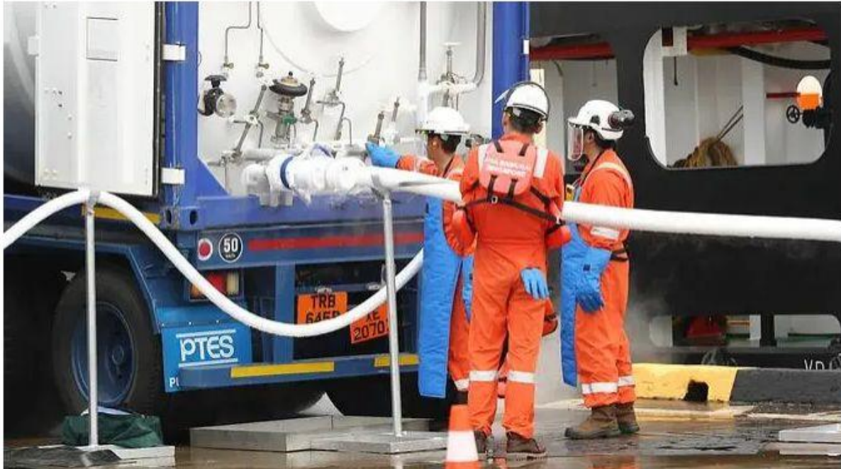
Workers carry out a bunkering demonstration, transferring liquefied natural gas (LNG) to a ship. (Photo: Pavilion Energy)
